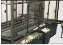
The optional enclosure is fabricated using a stainless steel frame structure with 3/8" thick polycarbonate door panels. The panels open easily to allow access to vials and when closed, they help reduce noise levels to below 75dB. The enclosure encourages consistent laminar flow and when combined with the lower air duct, it also enables a Hepa filtration system to be installed above the table to create a closed-loop drying system.
