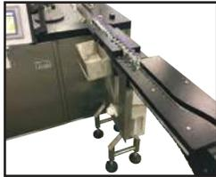
As the dried vial exit the machine in a single row, this device will reject any vials that are lying down. The vials are gently guided into a stainless steel bin which is lined with a soft rubber cushion.
