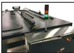
Andon lights come in handy because of their relative simplicity and their ability to be seen from a distance and attract the eye, especially in places where noise is high and other signals might not be noticed. Depending on the color that displays, workers can immediately rectify problems and get the production line moving again.
